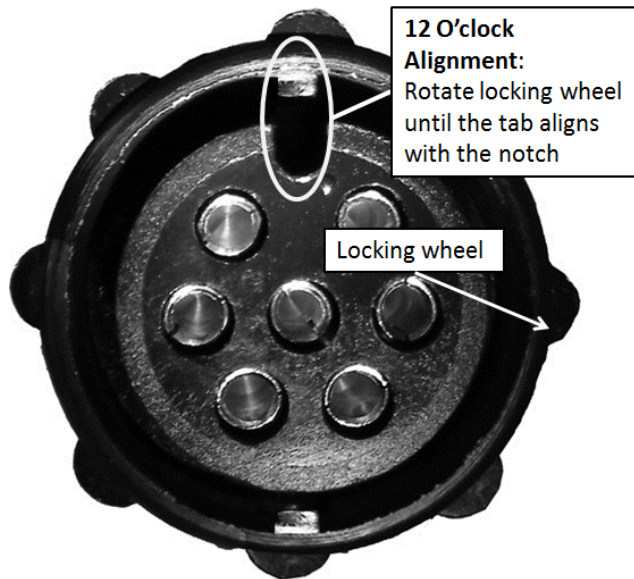
Figure 1 – Power port cable connector end-view
