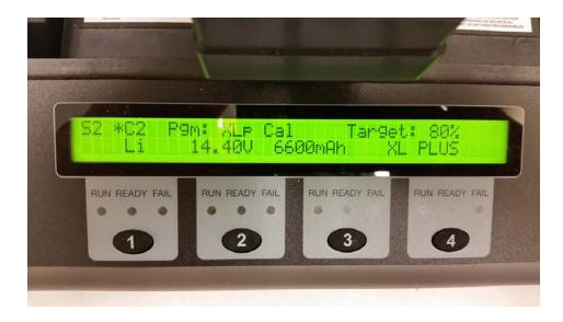
The XL+ adapter (PN# 07-111-5811) comes pre-programmed with C1 set to Charge. To set C2 to calibration the XL+ battery, enter in the following program and C-Code:
