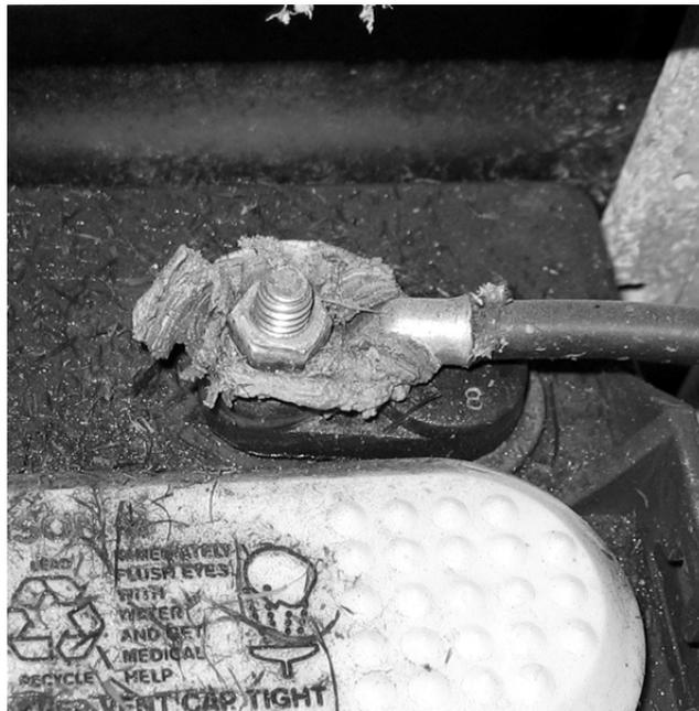
Figure 1: Example of Corrosion on a Battery Post
