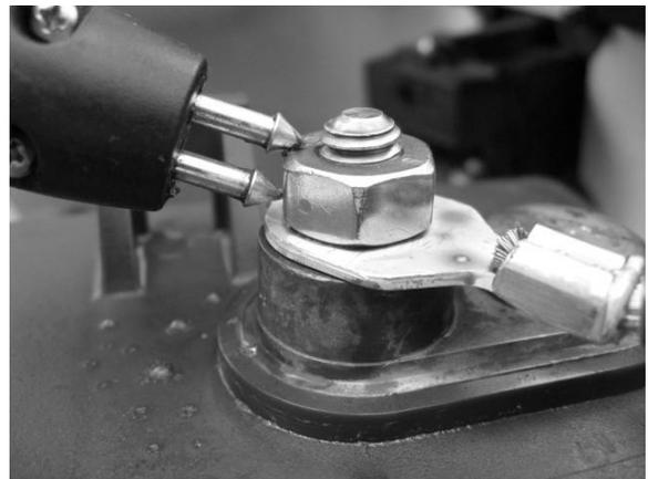
Figure 3: Probe incorrectly connected to the lead post
