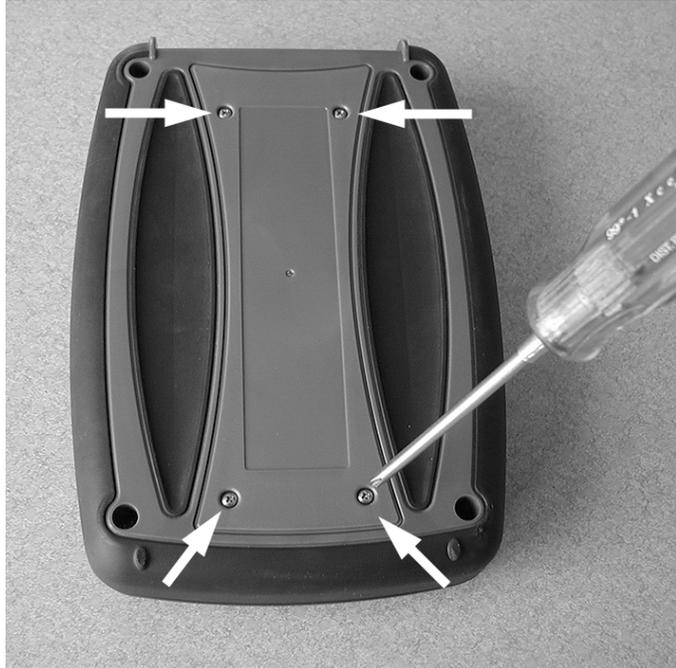
4. Remove the cover and locate the fuse adjacent to the battery connector.
