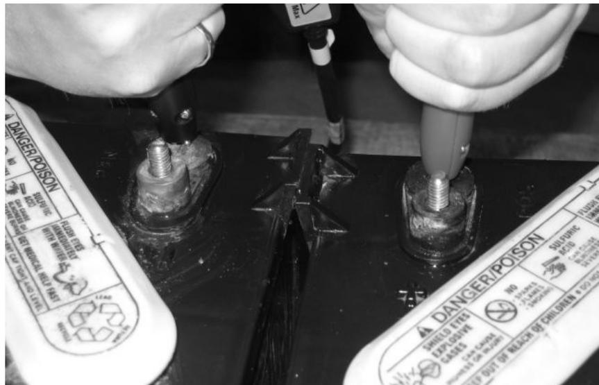
**Figure 7: An Incorrect Way to Connect Probes**
