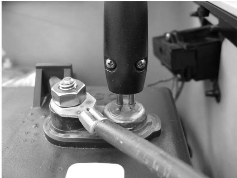
Figure 2: Probe is properly connected to the lead post
