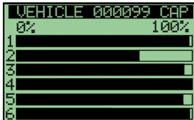
The Vehicle Capacity graph can help identify a bad or weak battery at a glance. The capacities shown are the estimated capacities each battery would have after a full charge.
