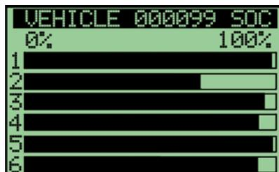
The **State of Charge** screen can help identify a battery that needs recharging or a set of batteries that need an equalization charge to bring the charge levels of all batteries to 100%.
