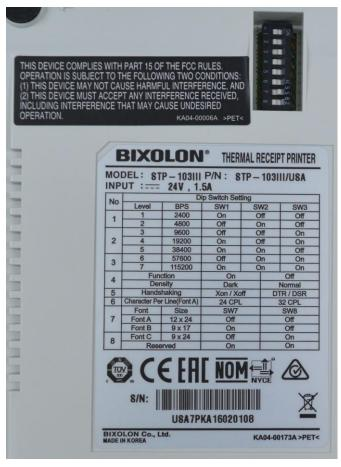
3. Follow the *Printer Installation Guide* that is included with the Bixolon STP-103 III thermal printer
